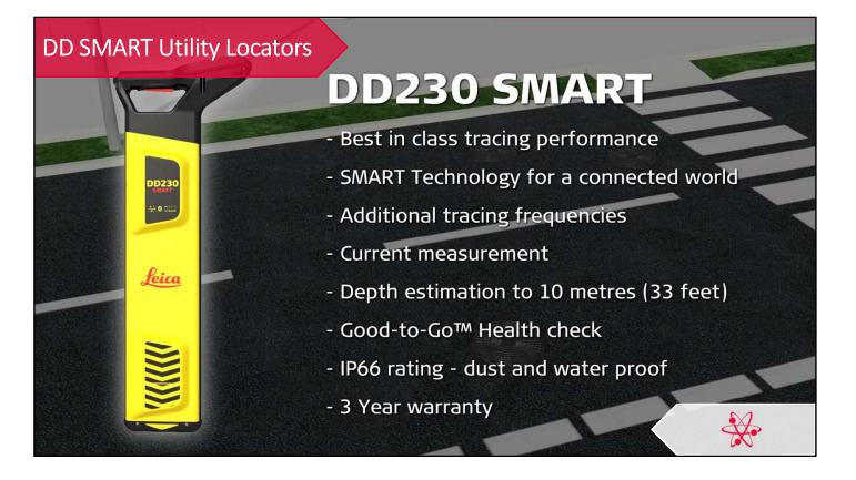
This follows the same protocol as the DD120 – DD130 and includes current measurement and two additional trace frequencies of 512Hz and 640Hz.
