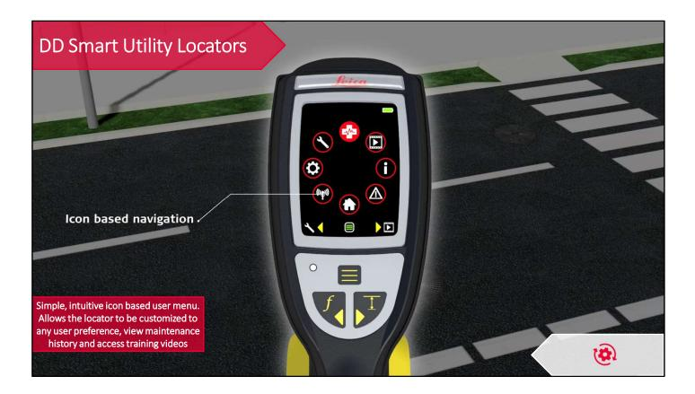
The built in icon based navigation menu allows setting to be changed quickly and easily more importantly, it allows fast access to the health check to ensure the locator is working properly to detect, locate, trace, or avoid utilities. The on-board videos are also accessed from this screen – NEXT SLIDE
