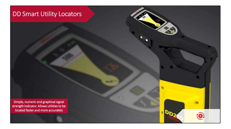
The Locators, both the DD100 & DD200 series, are fully automated. There are no controls to adjust while detecting utilities. The contractor simply walks forward, watches the bar graph rise (the yellow cone show). The systems also have a numeric and audio indication as well. When the highest number, bar graph reading, or audio is shown, this is then center of the utility.
