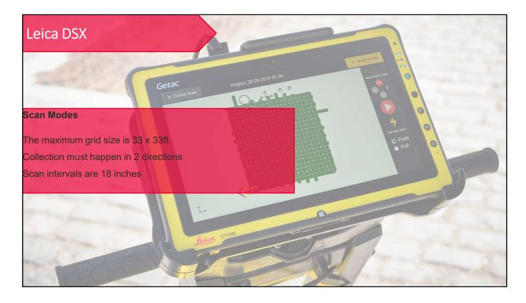
For the solution to work we need to collect data in a grid, the grid can be a maximum size of  $33 \times 33$  ft and as small as  $12 \times 12$  ft.
