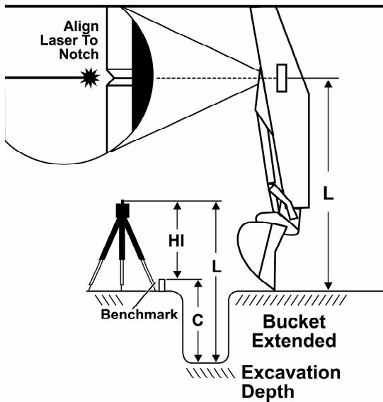
Place the laser in a location where receiver can pick up the beam, and turn it on.
