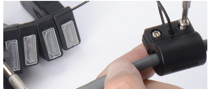
b. Holding them in place with your finger, turn clamp over and then place the Torx® screws into the holes and tighten down with the Torx® Pin Driver.
