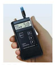
Ligno-VersaTec measuring relative humidity and temperature with the RH BluePeg Sensor
