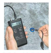
Ligno-VersaTec measuring the moisture in concrete with embedded RH BluePeg sensor
