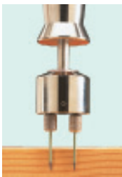
Slide-Hammer Electrode E12 surface / core
