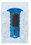
Moisture Testing in Concrete using in-situ Probes
