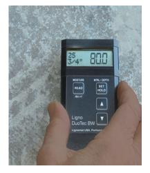
C Non-invasive meter for concrete D Non-invasive meter for wood
