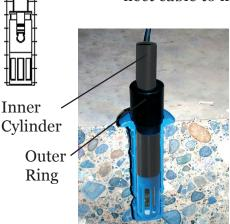
Remove Cable: Hold the inner cylinder in place with one hand and pull the end of the cable about 3/4" towards you. This disconnects the sensor from the cable. Now you can remove the cable-end-cover and the sensor will stay in the sleeve.
