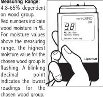
Wood Group Settings: The blue laminated card lists domestic and tropical species and corresponding wood group settings. Click on-off switch twice to check/change settings. Yellow LEDs indicate settings: 1-40 for wood (0 and 41 is for building materials). Click on-off switch again to change setting. Check/Change Mode is only accessible when meter is off. If a wood species is not listed on the laminated blue card, contact customer service at 800-227-2105.
