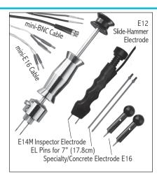
**E12 Electrode** and mini-BNC Cable is for measure- ments up to 2" (50mm) deep in wood and soft building materials (drywall, gypsum, plaster, etc.) Allows comparing surface and core moisture.
