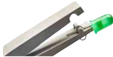
RX 601 forming pliers leave a standoff on the LED leads.
