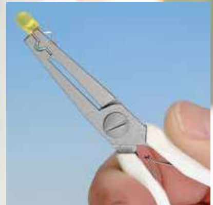
341A cut and form pliers put stress relief in component lead and trims to length with one squeeze.
