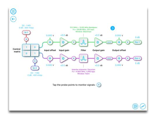
Sampling Rate Up to 39.06 MHz Filter Coefficients Up to 14,819
