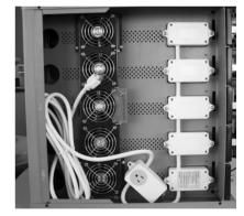
If no pedestal is being used under the stack, plug the top FUYL Cell into the 'hidden' socket - located inside the left cover of the FUYL Cell below.
