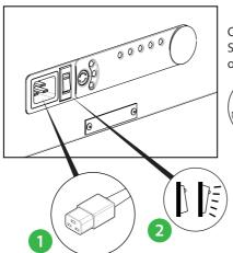
Connect the power cord and switch on. Use ECO Safe Charge $^{\text{m}}$  instructions (included in the box) for operating details.
