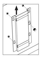
Loosen the thumbscrew and slide keyholes over the studs to remove the cable management cover.
