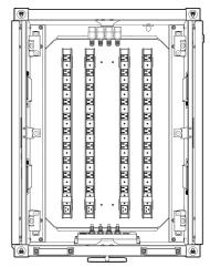
Relocate Power Distribution Units as desired. Arrange devices' power adaptors in the base of cart
