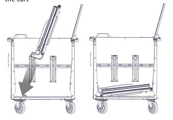
Push the tray forward so the face is flush with the side panel
