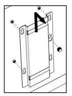
Loosen the thumbscrew and slide keyholes over the studs to remove the cable management cover.
