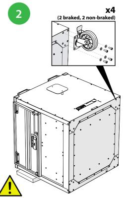
Use a piece of packing foam for protection when carefully laying down the cart
