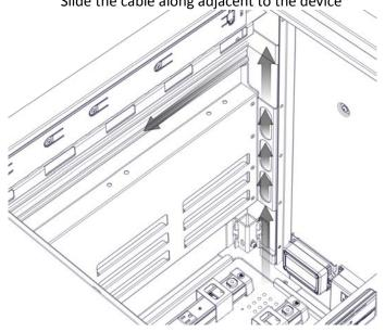
Insert the remaining cables. Evenly space the cables along the rubber grip
