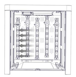
Run the cable up through the hole at the end Pull the cable through the rubber grip. Slide the cable along adjacent to the device
