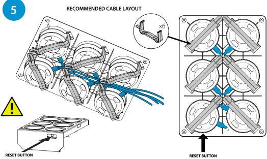
Adjust the Sphero charging base to allow access for the reset button through the access hole.
