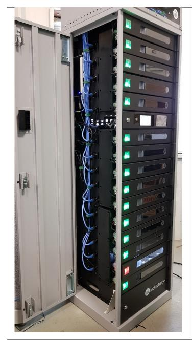
All 15 lock modules are now accessible. Locate the lock module for the bay you wish to override and open
