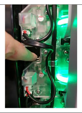
Firmly press down on the lever on the top left of the lock module to release that door.
