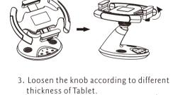
4. Press the clips by hands to accommodate Tablet with different dimensions(7"~10.1")
