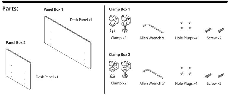
1 Please read all instructions before installation. Choose the desired height of the Panel. Hold Clamp up to the pre-drilled hole and insert Screw through the Clamp and into the Panel. Make sure that the Clamp is straight up and down for proper attachment to desk. Use the Allen Wrench to tighten until secure. Repeat with the other Clamp.
