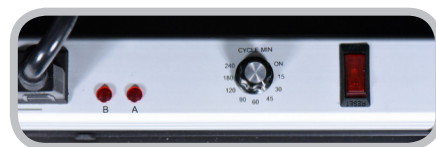
Timer for charging cycle control
