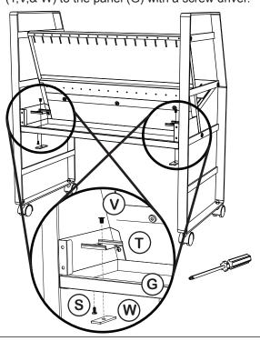
Step 7: Push the power strip (X) into the brackets.
