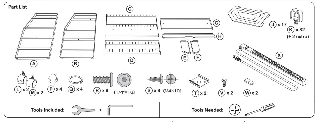
Step 1: Attach the casters (L & M) to the side frames (A & B) with the lock washer (Q) and acorn nut (P), using the included wrench.
