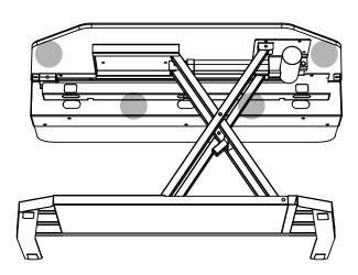
Step 3: Attach the provided cable clips on the underside of the unit. Place items on the desk and run cables through the clips. Check cables for slack and pinch points.
