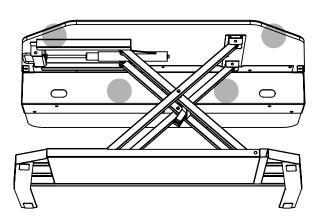
**Step 3**: Attach the provided cable clips on the underside of the unit. Place items on the desk and run cables through the clips. Check cables for slack and pinch points.
