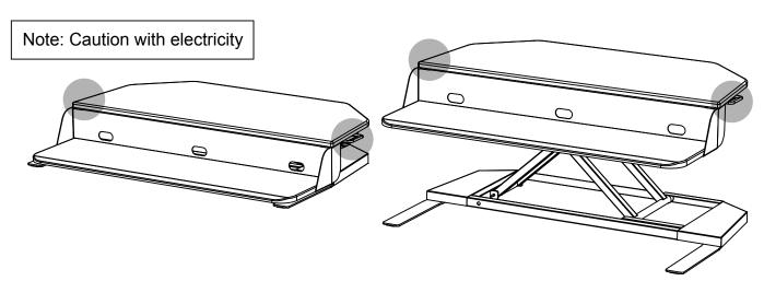
**Step 1**: Squeeze the handle on the underside to raise the unit. Lift with hands on both sides.
