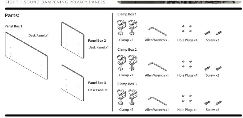
(1)Please read all instructions before installation. Choose the desired height of the Panel. Hold Clamp up to the pre-drilled hole and insert Screw through the Clamp and into the Panel. Make sure that the Clamp is straight up and down for proper attachment to desk. Use the Allen Wrench to tighten until secure. Repeat with the other Clamp.
