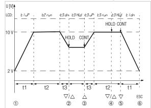
**Ramp parameters:** output quantity: U (range of 0 ... 15 V), 5ERrt = 2 V, Ernd = 10 V, t = 5 s, t = 8 s, t = 5 s, repeat for periodic ramps
