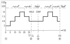
**Interval parameters:** output quantity: U (range of  $0 \dots 15$  V), St.Rrt = 2 V, End = 10 V, number of interval StEP5 = 3, E I = 5 s, NadE = Ruta
