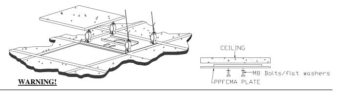
The ceiling should be capable of supporting a weight of at least five times the projector or monitor weight. If it cannot, the ceiling must be reinforced. Proper installation procedure by qualified personnel as outline. In the installation instructions must be adhered to. Failure to do so could result in serious personal injury. For further information or ordering assistance contact us at the address shown on the front of this page.
