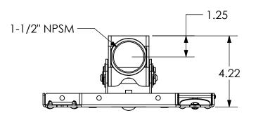
NOTE: CUSTOM INTERAFCE BRACKET NOT SHOWN. THE CUSTOM INTERFACE BRACKET NEEDED FOR YOUR DISPLAY WILL ADD BETWEEN 1/2" AND 2" IN DEPTH AND MAY AFFECT LOCATION OF DISPLAY ON THE MOUNT.
