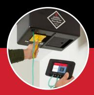
The Exhaust Fan Flow Meter. shown with the DG-700, is used to measure airflow through bathroom fans, whole house ventilation fans and other exhaust devices.
