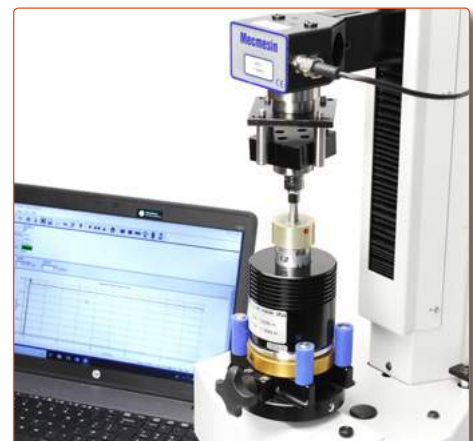
Torque value check on Helixa
