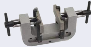
Shown fitted with a half-set of Mec240g-BD80 diamond jaws.
