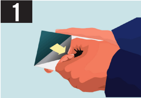
1 Peel the white protective coating off of your Presensitized Copper Clad Board (600 Series)
