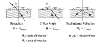
In the MA872, light from an LED passes through a prism in contact with the sample. An image sensor determines the critical angle at which the light is no longer refracted through the sample. The MA872 automatically applies temperature compensation to the measurement and converts the refractive index of the sample to Fructose concentration in units of percent (by weight).
