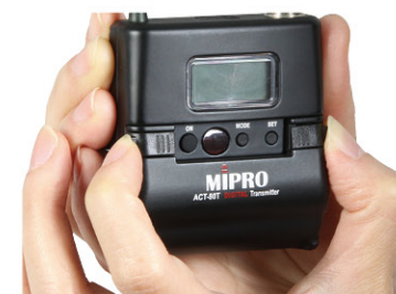
Squeeze and hold battery levers
