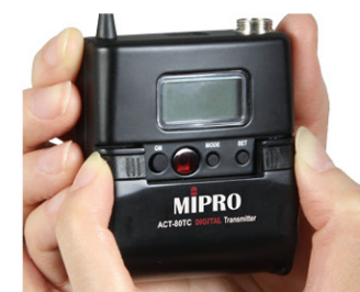
Squeeze and hold battery levers
