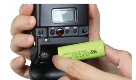
Insert or remove battery
