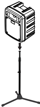
Installed on a tripod
