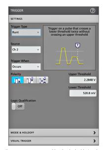
Figure 8: Configuration menus are accessed by simply double-tapping on the item of interest on the display. In this case, the Trigger badge was double-tapped to open the Trigger configuration menu.
