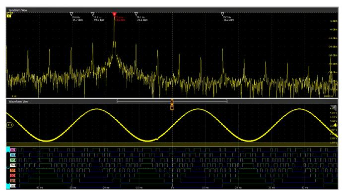
Figure 5: Beyond just analog and digital, FlexChannel inputs include Spectrum View. This Tektronix-patented technology enables you to simultaneously view both analog and spectral views of all your analog signals, with independent controls in each domain.
