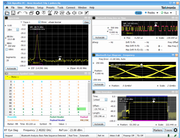
Easy validation of Bluetooth transmitter with push button preset, pass/fail information and clear correlation between displays.
