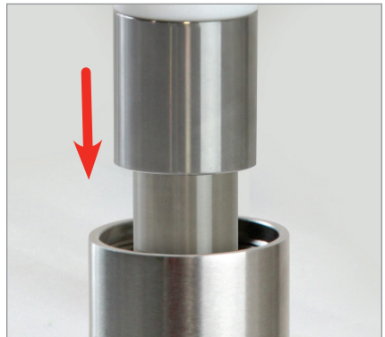
4. Slide the data logger and lid back into the barrier body and screw the lid back on tightly.
