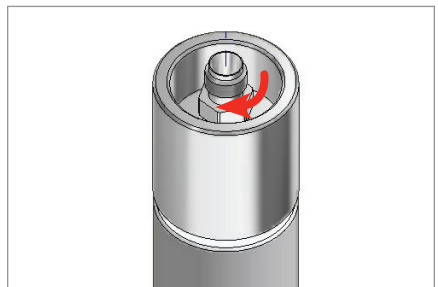
2. Screw the Fitting Body into the end of the stopper assembly (finger-tight).
