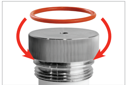
2. Stretch the O-Ring over the endcap so it sits in the groove just beneath the knurled shoulder.
