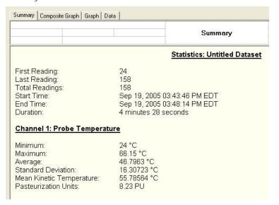
In this example, the process was exposed to 8.23PU. With these MadgeTech tools, you can build an understanding of the relationship between the process temperature and the amount of time exposed to the process without the headache of spreadsheets and formulas.
