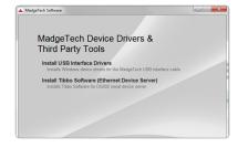
The default directory is C:\Program Files\MTI-USB\Datalogger Interface. If you choose to change the location of the install directory, select the Change Install Location button. Once you have the install location set select the Install button to start the installation.
