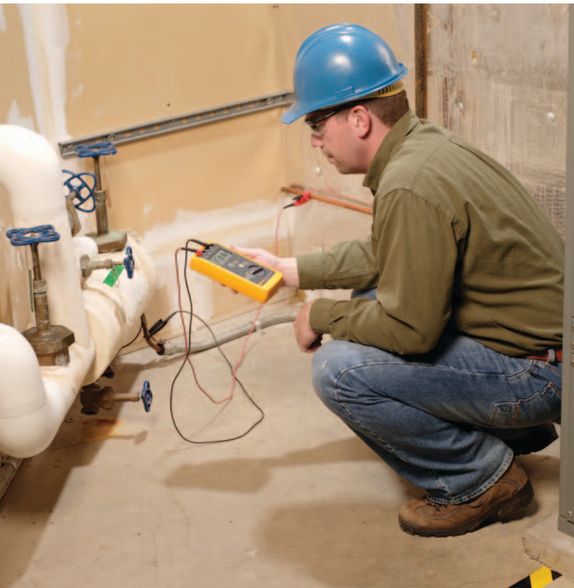
The Fluke 1621 Earth Ground Tester is an easy-to-use earth ground tester, the first line of defense in detecting reliable ground connections.
