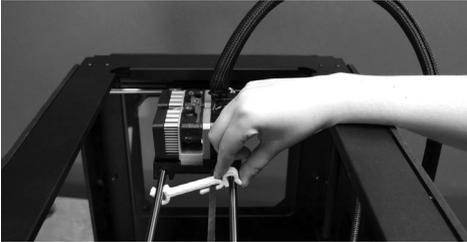
3b. A small plastic piece attached to the X-axis belt and gantry rods prevents the extruder from moving. Carefully snap the piece off of the rods and tilt it to slide it off of the belt.
