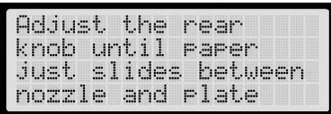
Adjust the rear knob until paper just slides between nozzle and plate
