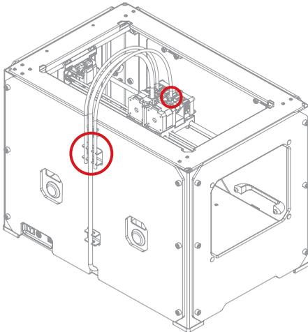
5a. Locate the two filament guide tubes. Insert one end of a filament guide tube into the hole in the top of one of the extruders. Push the filament guide tube in as far as it will go. Insert the end of the other filament guide tube into the hole on the top of the second extruder. Push the filament guide tube in as far as it will go.
