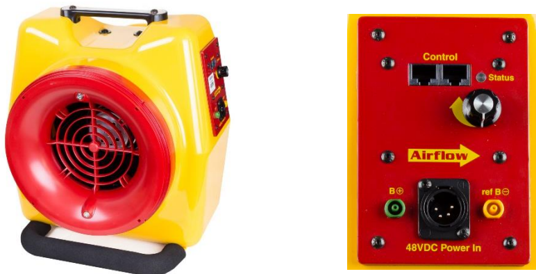
Figure 4: Retrotec Model 300 has a speed control knob and two Ethernet style Speed Control Ports for daisy chaining speed controls for running many fans together. Tubing connections to the gauge, both color coded, are shown.
