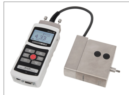
FS05 force sensor connected to an M5I indicator via AC1083 adapter for off-site calibration
