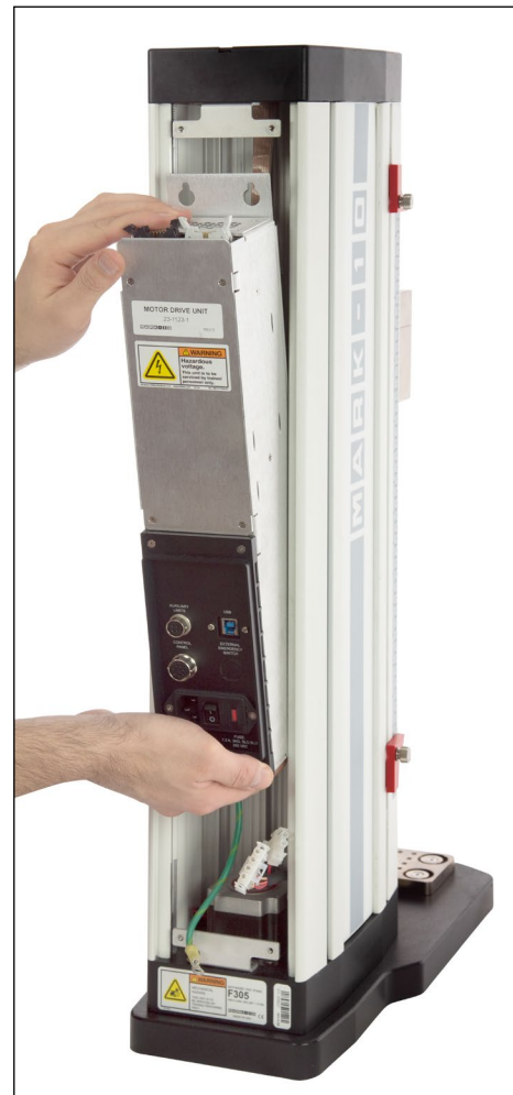
Removing the MDU
