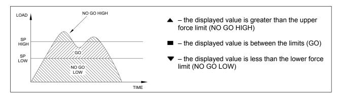
**Note:** Set point indicators and outputs reference the displayed reading, not necessarily the current live load.
