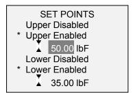
One, two, or none of the set points may be enabled. To toggle between the tension and compression directions, press the **DIRECTION** key.
