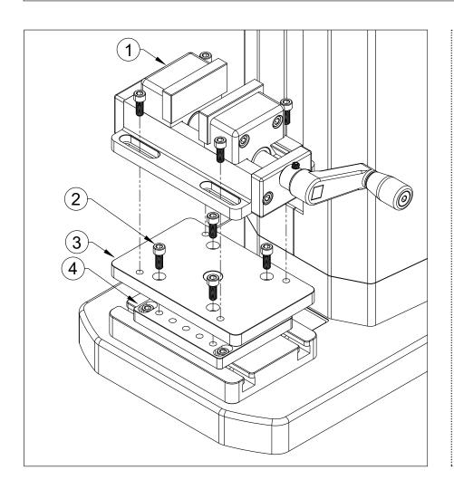
The G1106 vise grip is designed to secure test samples for various compression and tension measurement applications. It may be mounted to Mark-10 test stands with a 25-hole base plate, such as pictured at left.
