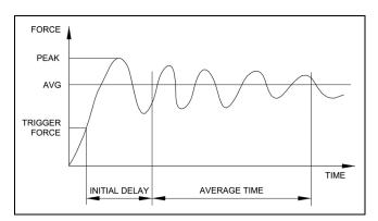
2. Averaging occurs only while above the trigger force. As the force drops back down to this trigger, averaging stops. To enable this function, scroll to **Stop at Force** and press **ENTER**.
