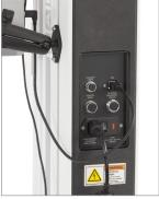
Connect the included USB cable between the USB-C port and the USB-B port in the rear of column, and connect the AC adapter connector.
