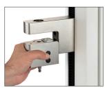
Series FS05 force sensors mount directly to the crosshead. Match the gold-plated pads on the top surface of the load cell block with the pins in the underside of the crosshead, as shown at left.
