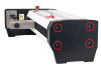
The end cap is shipped in a separate box within the main box for the Model F505H test frame. Line it up with the right end of the column, then install with the four included screws, as shown at left.
