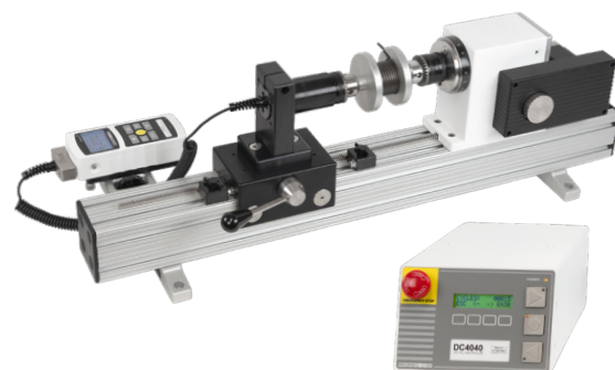
^ Model TSTMH-DC is shown in a torsion spring test, with a Series R50 torque sensor and M5i force/torque indicator
