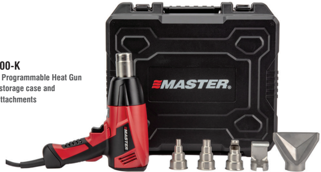
Programmable Backlit LCD Display Variable Temperature in 10°F increments (5°C) 9 Airflow Settings 4-18 CFM 4 Preset Programs Selectable Auto Cooldown Feature Supervisor Locking Feature
