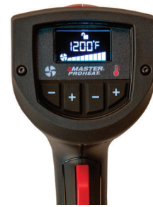
Programmable Backlit LCD Display Variable Temperature in 10°F increments (5°C) 9 Airflow Settings 4-18 CFM 4 Preset Programs Selectable Auto Cooldown Feature Supervisor Locking Feature
