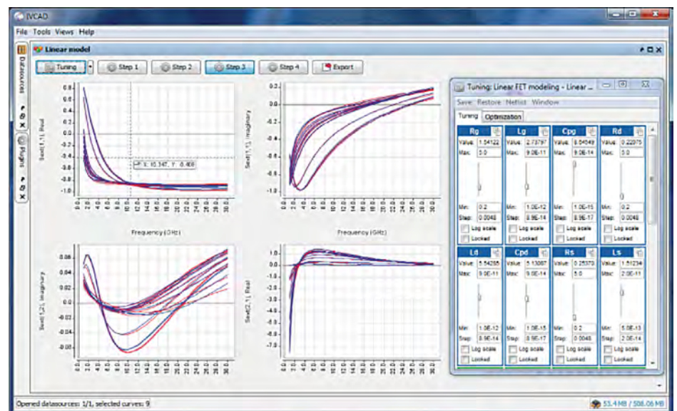
Linear Model Comparing Measured And Optimized Data
