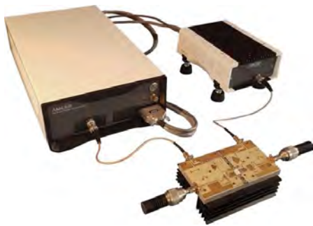
AM3100 used for pulsed bias of Power Amplifiers
