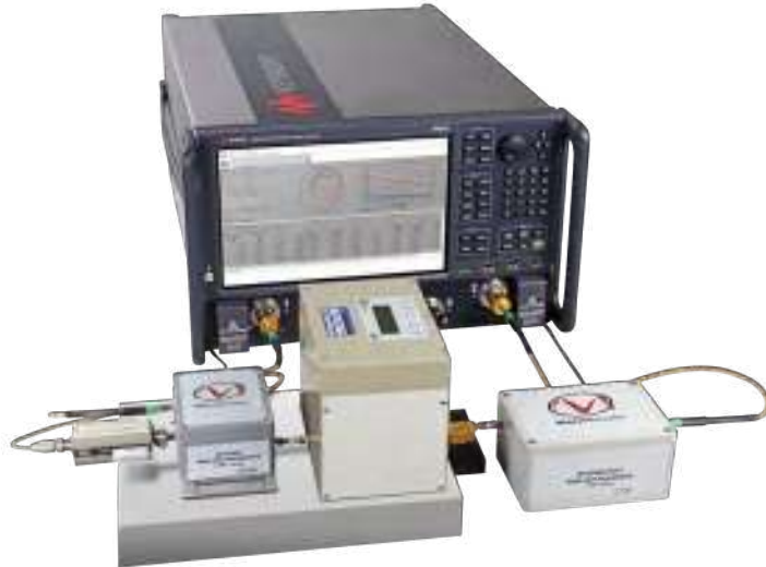
Typical setup for performing high-speed noise parameter measurements.
